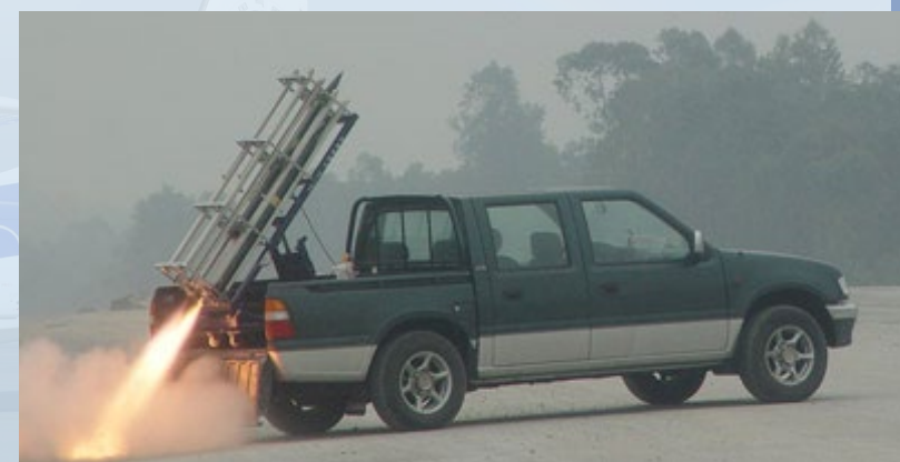
人影火箭发射架及火箭发射 Weather modification rocket launcher and rocket launch
